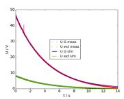
During breaking, the first motor on the left is disengaged. Its voltage (UG) serves as a measure of the angular velocity of the wheel. The second motor is engaged: it acts as a generator whose voltage (Uext) is measured across the external load resistor; it drives the flow of electric charge. Fitting simulation results to dynamical data yields values of missing parameters.
