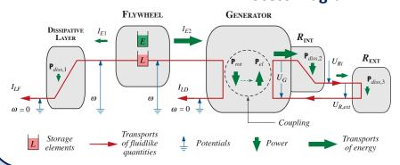
Process diagrams visualize explanations of physical processes—they show storage and flow of fluidlike quantities and energy and introduce power as the measure used in the coupling of processes. Here, the generator couples mechanical and electric processes.
