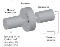
An electric DC motor/generator (on the right) is attached to a flywheel. The spinning wheel drives the device as a generator that is connected to an external electric resistor to form a single-loop circuit. As the flywheel spins down, voltages and angular velocities are measured with the help of the motors/generators on the left and on the right.
