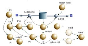
A dynamical model based upon the balance of angular momentum (L) of the wheel. The braking moment (I L damping) of the motor/generator is calculated indirectly via the electric power (P el) of the generator leading to an *electromechanical feedback loop* in the model: We use the notion of *power of processes and its balance* in the coupling of different types of processes. This constitutes a *direct and indispensable application of the energy principle*.
