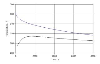
Figure 7: Data taken during the cooling of hot water in a thick walled PVC container (upper curve: water; lower curve: surface of container).
